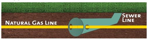
A blocked sewer line may be the result of another utility line (gas, electric, telecommunications) accidentally cross boring through the sewer line. A cross bore is an unsafe intersection of two different utility lines. Do not try to clear a sewer line blockage yourself. It could result in a serious accident. The safest way to ensure there is no cross boring in your sewer line is to have a plumbing professional inspect the line with a video inspection system.
